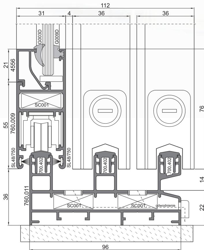
**A non-insulated aluminium profile system designed for the construction of internal and external joinery, including sliding partitions and balcny constructions**
