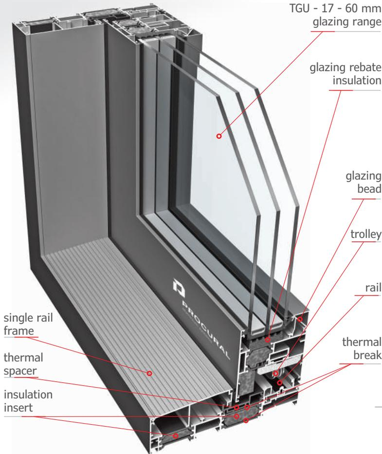
**A sliding system with insulated profiles designed for the construction of external joinery.**
